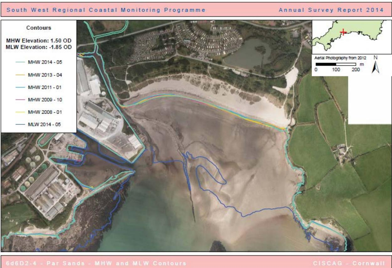
Figure 3.8 MHW contour change at Par Sands (source: PCO, 2014a).
