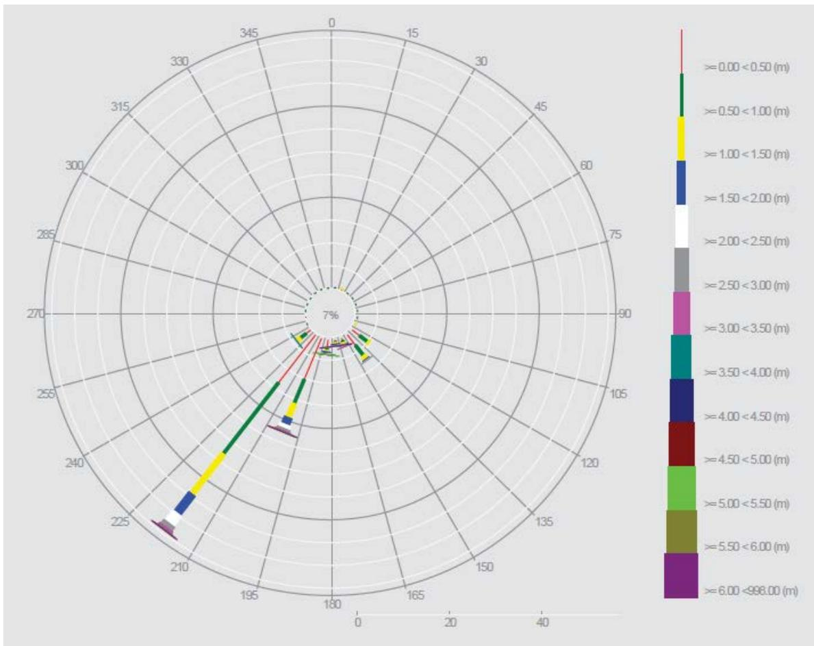
Figure 3.1 Offshore wave height recorded by the Looe Bay Directional Waverider Buoy between 22nd June 2009 and 30<sup>th</sup> June 2014 (PCO, 2014a).
