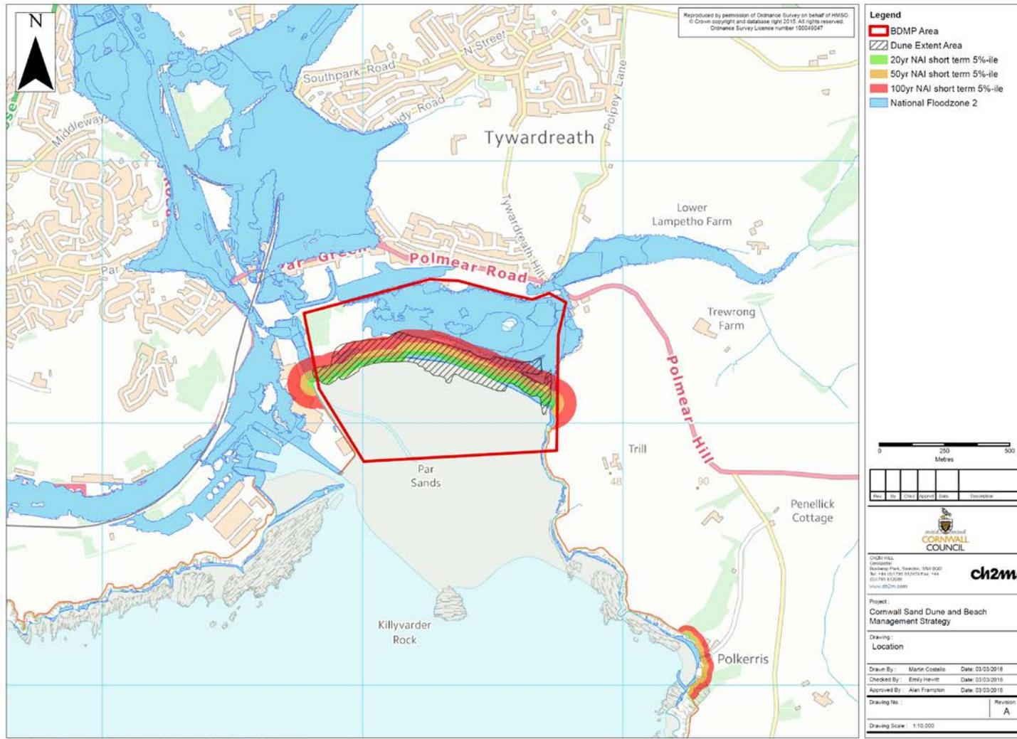
Figure 3.11 Flood and erosion risk projections for Par Sands.
