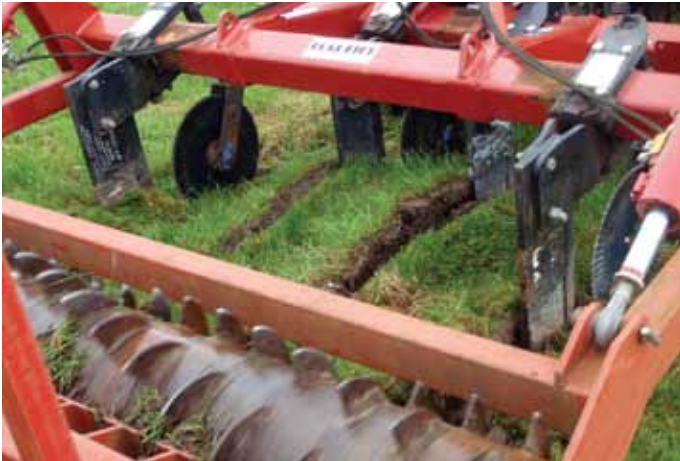
A sub-soiler for reducing runoff from agricultural land
